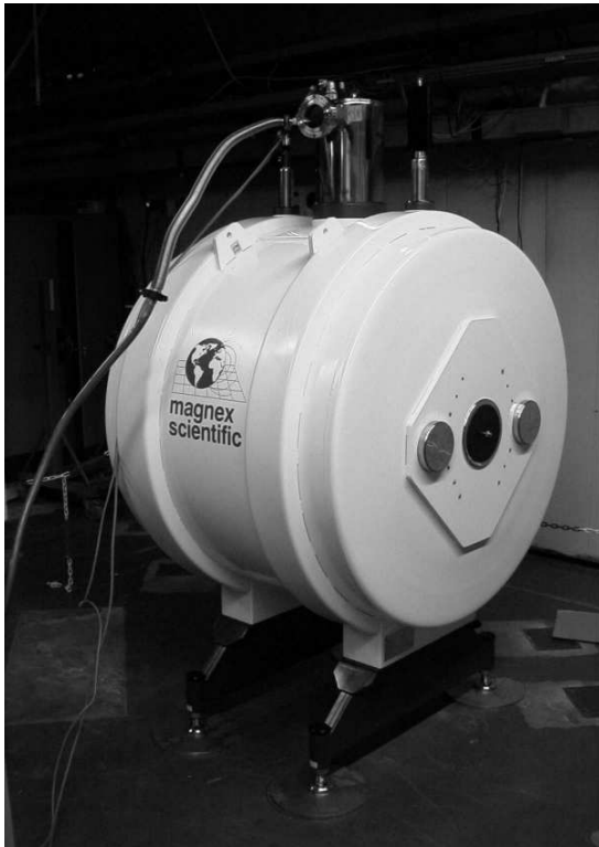
Fig. 1. The 7 T superconducting magnet with two homogeneous field centers for the operation of the double-Penning-trap system.
