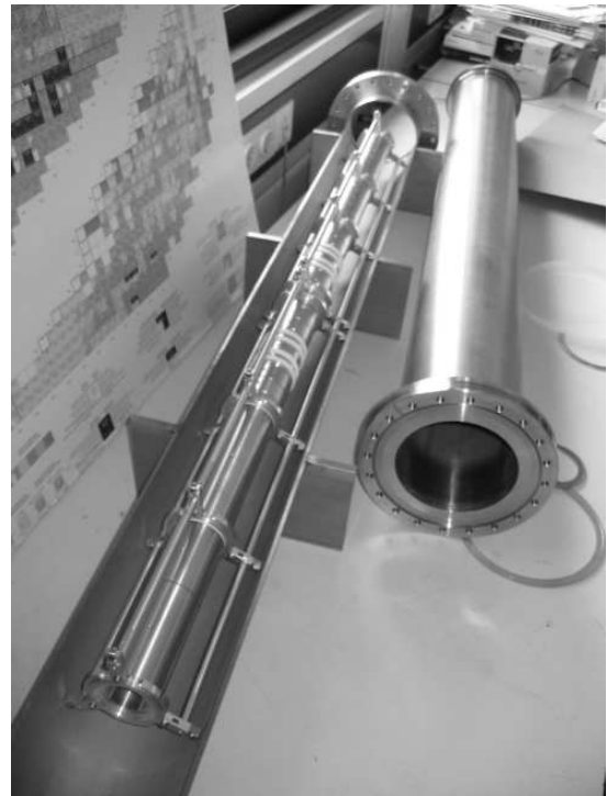
Fig. 2. Electrode structure of the double-Penning-trap system.
